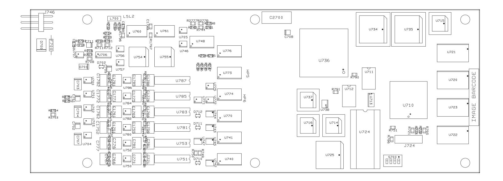
Figure 6-16. DSP Assembly, Component Locations (sheet 1 of 2)
