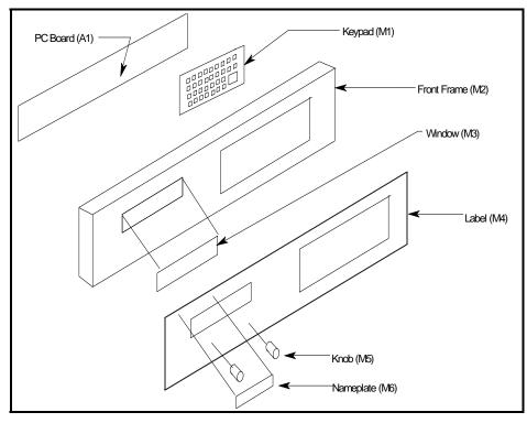
Figure 5-1. Front Panel Components (see Table 5-1)
