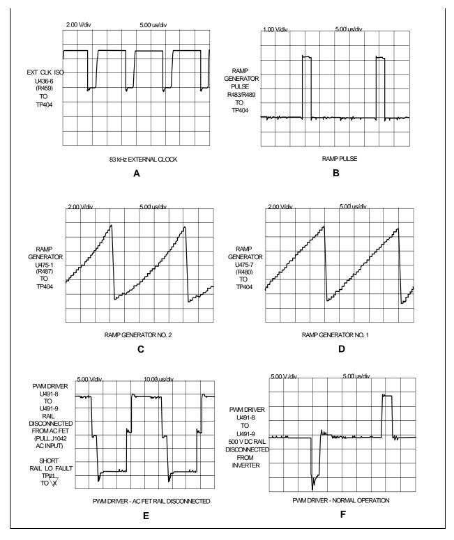
Figure 4-5. DC Rail Assembly - Test Waveforms
