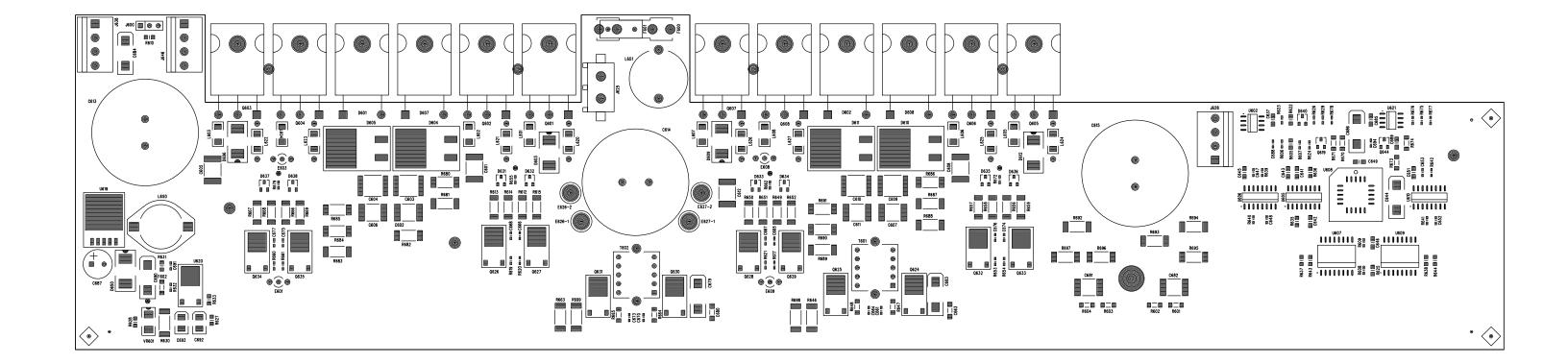
Figure 6-14. Inverter Assembly, Component Locations
