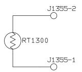
Figure 6-25. Thermistor Assembly, Schematic Diagram
