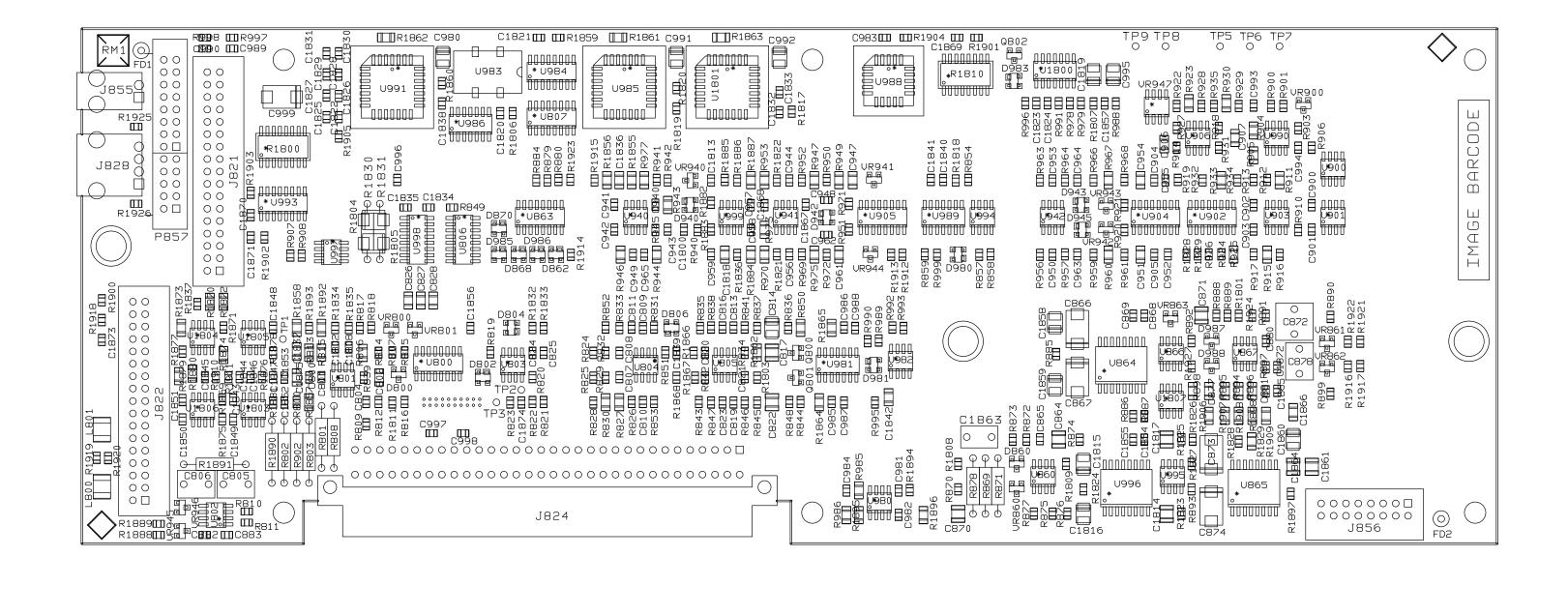
Figure 6-18. Control Board, Component Locations (sheet 1 of 2)
