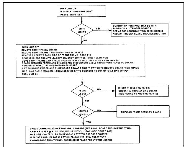
Figure 4-2. Front Panel Assembly Troubleshooting
