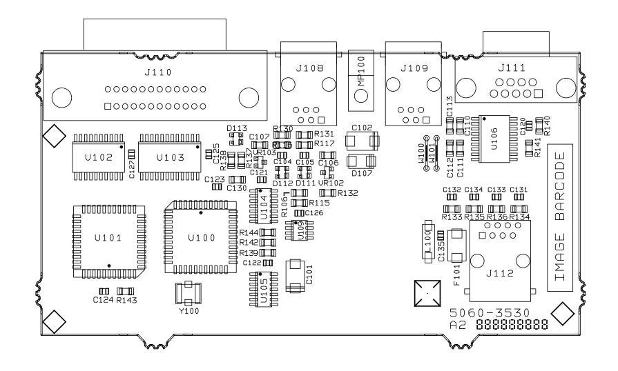
Figure 6-4. GPIB Assembly, Component Locations
