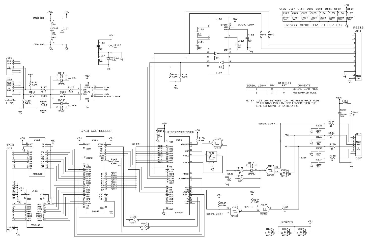
Figure 6-5. GPIB Assembly, Schematic Diagram
