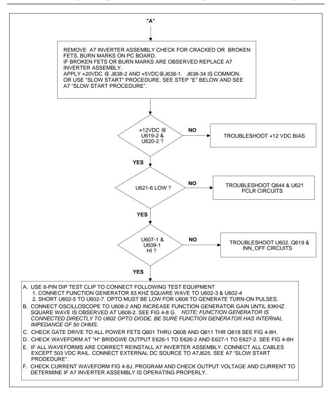
Figure 4-7. Inverter Assembly Troubleshooting (sheet 2 of 2)
