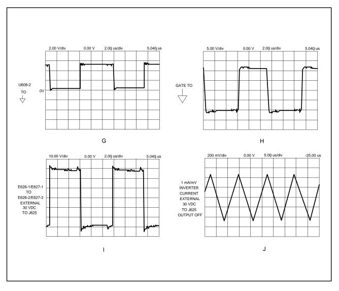
Figure 4-8. Inverter Assembly - Test Waveforms (sheet 2 of 2)
