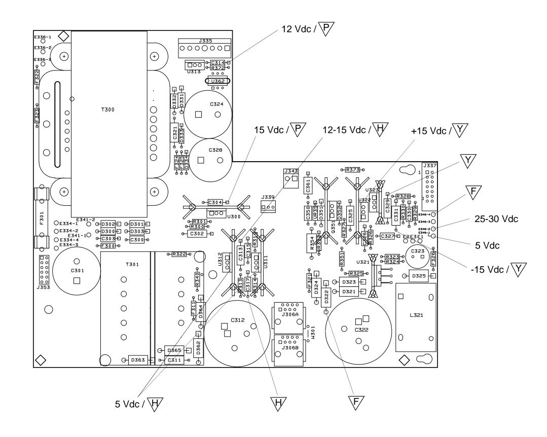
Figure 6-12. Bias Assembly, Component Locations
