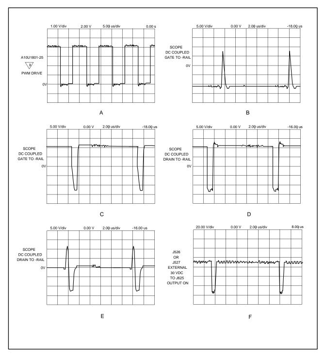
Figure 4-8. Inverter Assembly - Test Waveforms (sheet 1 of 2)
