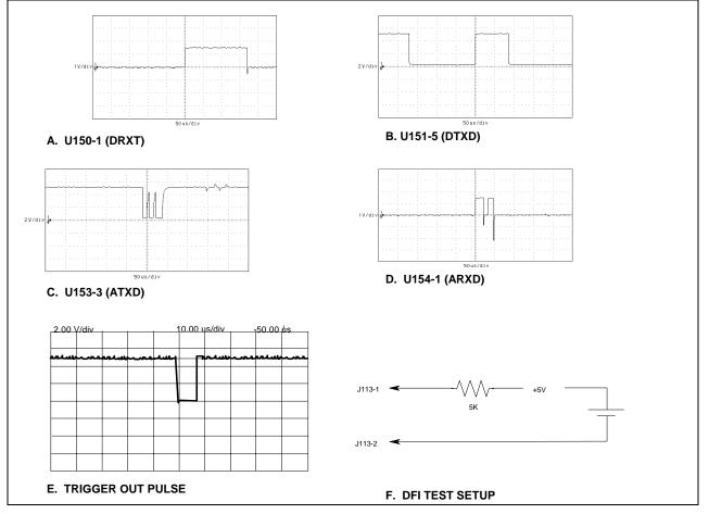
Figure 4-10. Trigger/BNC Assembly - Test Waveforms
