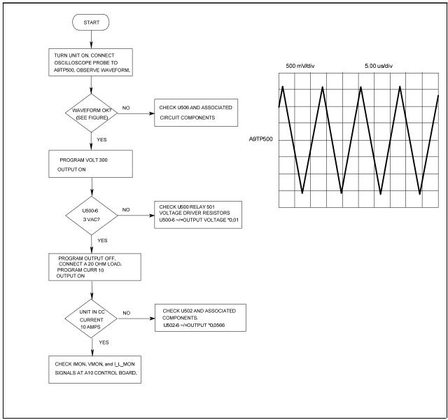
Figure 4-9. Output/Filter/Relay Troubleshooting
