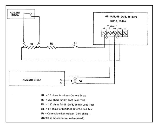
Figure 2-1. Test Setup
