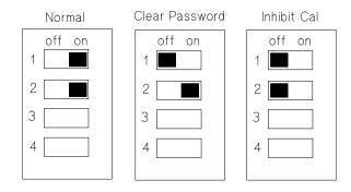
Figure 4-11. Calibration Switches
