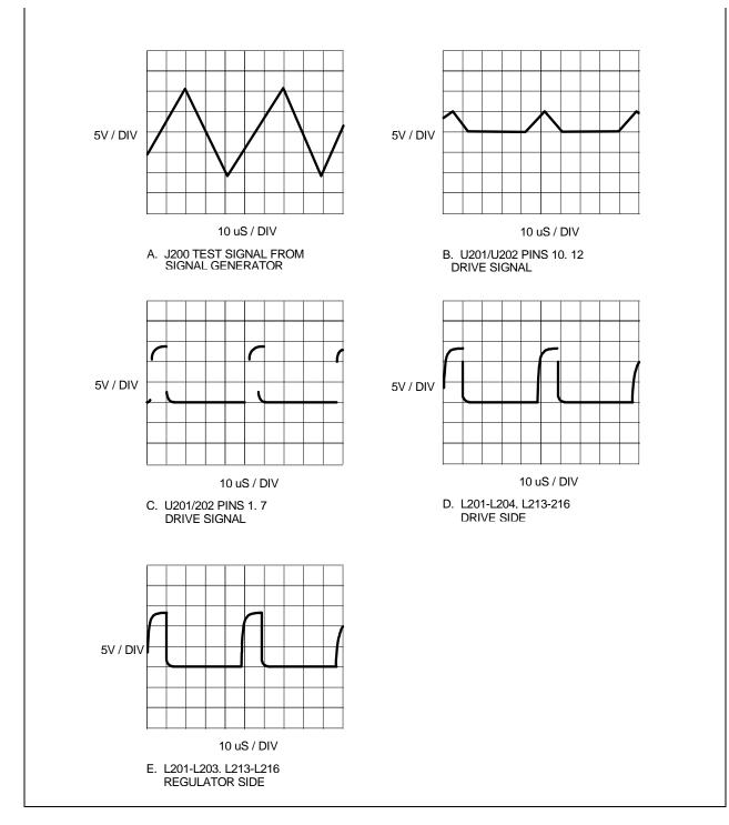
Figure 4-3. FET Assembly Test Waveforms
