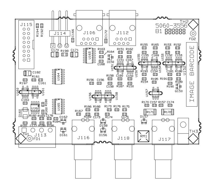
Figure 6-22. Trigger Board, Component Locations
