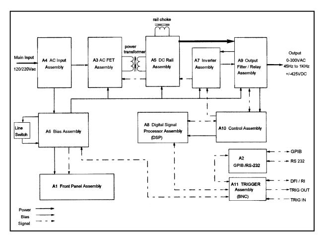
Figure 3-1. AC Power Source/Analyzer Block Diagram
